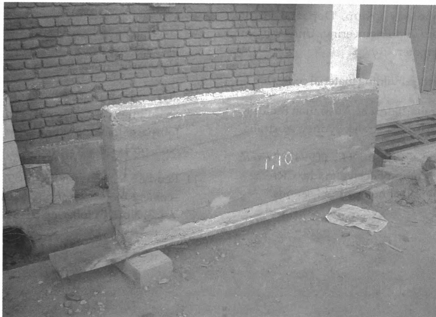
Figure 4: Wall panel used for flexural testing
