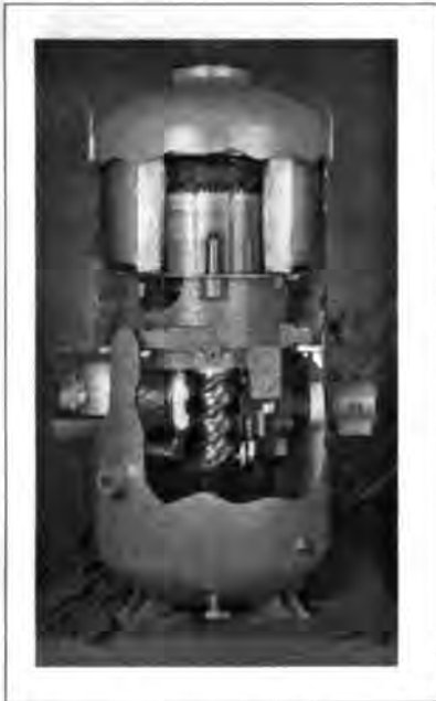
Fig.3 Vertical Hermetic Screw Compressor used in chiller packages (Courtesy of Dunham-Bush)
