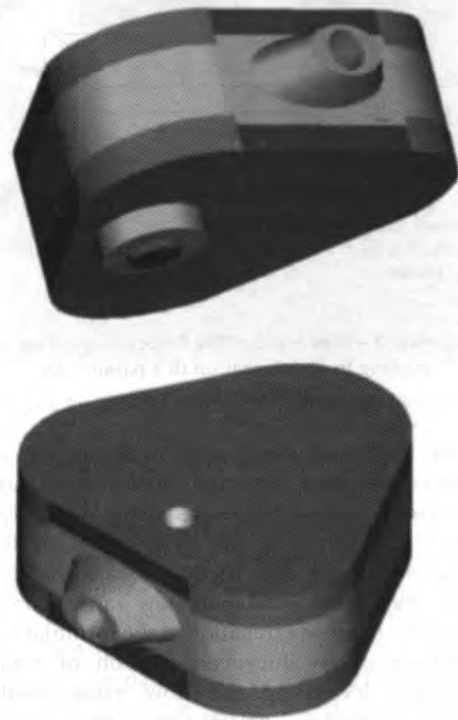
Figure 3 - Assembled Geometrical Model of the Third Multi-Dose Inhaler
