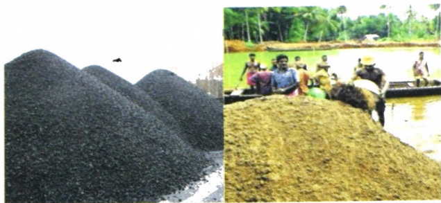
Usual coarse aggregate (Crushed stones) and fine aggregate (River sand) for concrete
