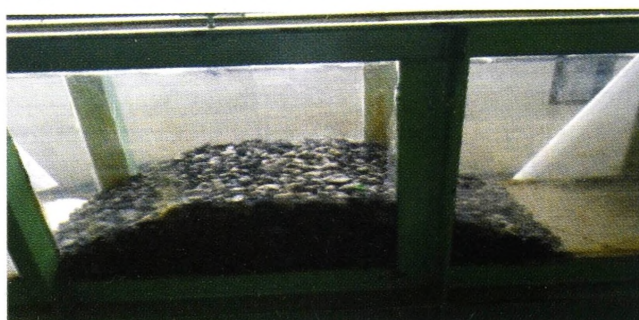
Figure 3 - Breakwater model of 40 cm crest width using 26 mm armour units
