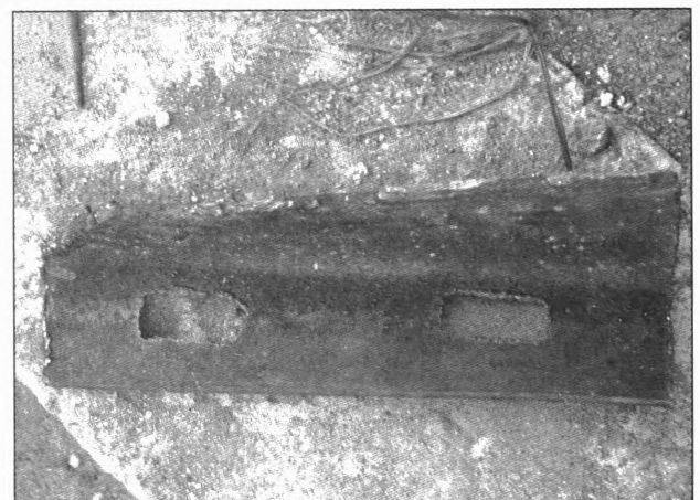
Figure 7. Flame Cut Angle Bracket
