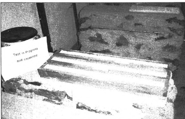
Figure 12: Shrinkage test mould filled with soil
