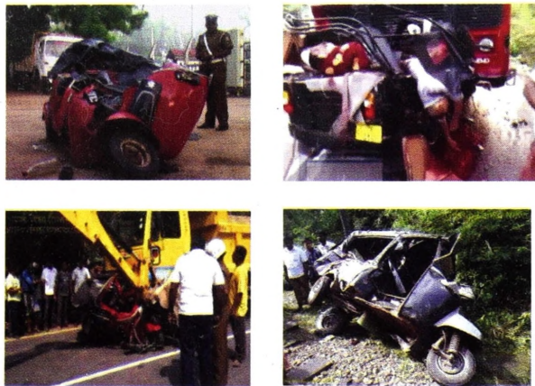
Figure 2 - Three wheeler accidents due to hitting while tending for toppling-Toppling condition is evident from the damages to hood
