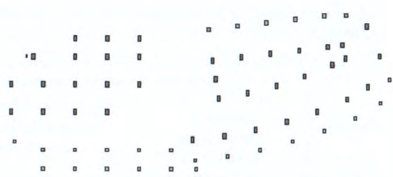
Figure 3 - Wrong column orientations when default values are used
