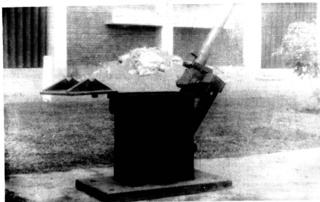
Figure 1 (a) 'CINVA' ram - Machine ready to accept the cement-sand mix (catch at the junction of two lever arm sections engaged)
